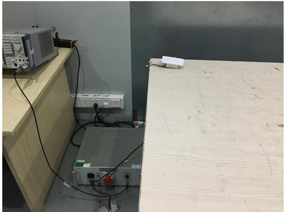
Conducted Emission Test Setup
