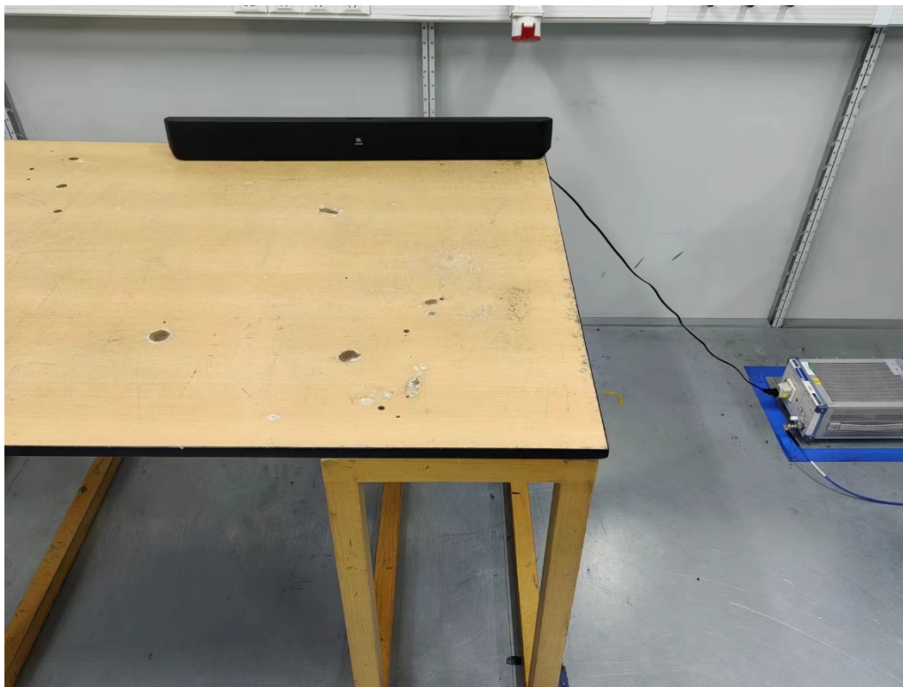
Photograph 3: Set-up for Conducted Emission on AC Mains
