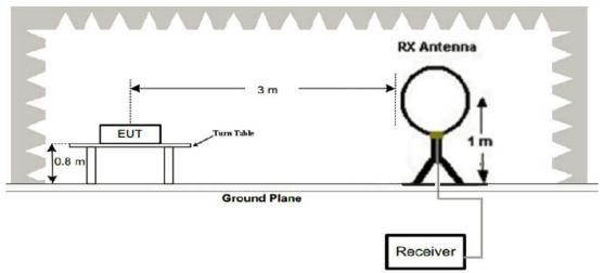
(2) Radiated Emission Test-Up Frequency 30MHz~1GHz
