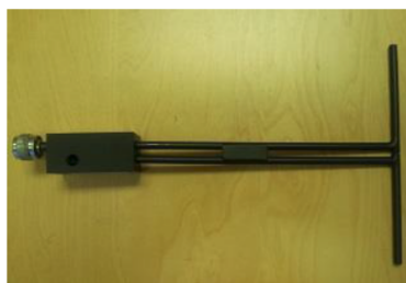
Figure 1 – MVG COMOSAR Validation Dipole
