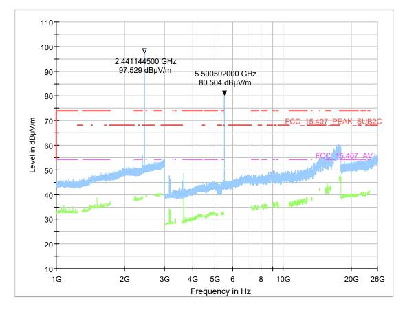
Remark: The two peaks (above the limits) are the wanted signals at the carrier frequencies.
