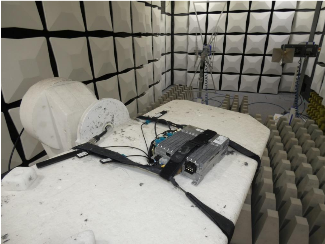
Photo 1: Test setup for radiated measurements (Enclosure, fully-anechoic chamber, 1-26 GHz intentional radiator §15, ANSI C63.10)
