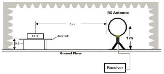
(2) Radiated Emission Test-Up Frequency 30MHz~1GHz
