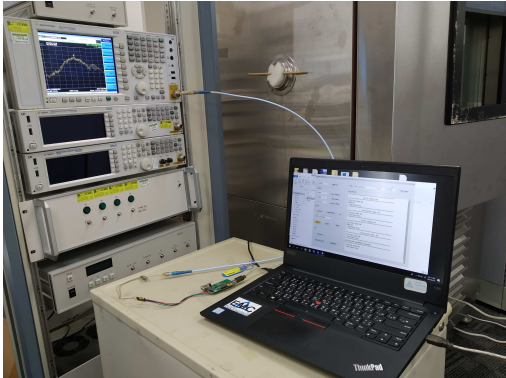
Photograph 4: Set-up for Conducted testing
