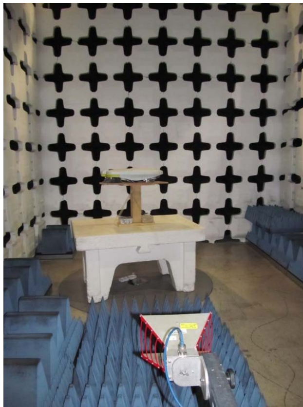
Radiated emissions test setup with Horn antenna.
