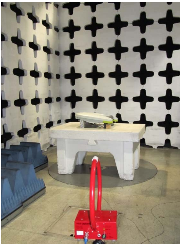
Radiated emissions test setup with Loop antenna.
