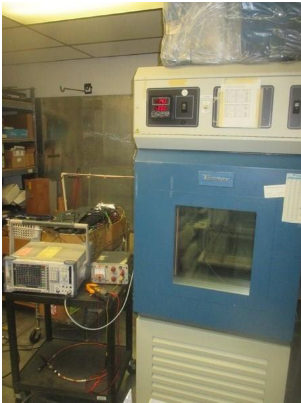
Figure 3.4 Frequency Tolerance Test Setup
