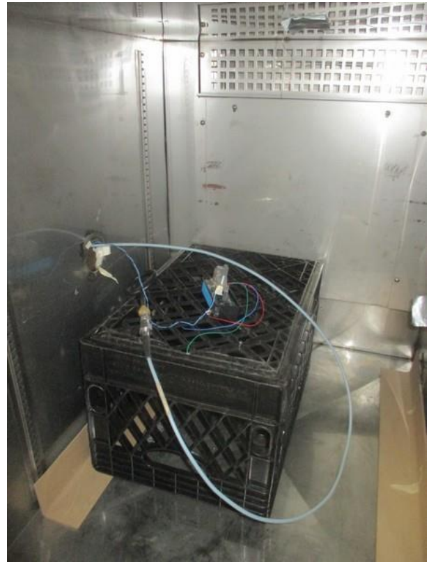
Figure 3.4 Frequency Tolerance Test Setup
