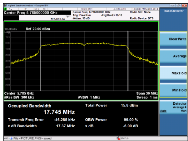
(802.11 AC20) 6dB&99%Bandwidth plot on channel 165
