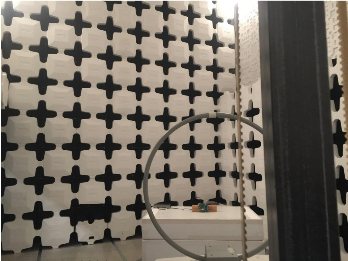
Figure 2. Loop Antenna, below 30 MHz Testing
