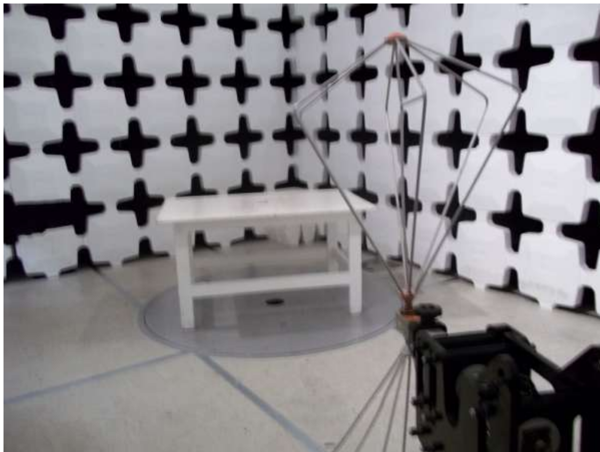
Figure 3. Radiated Emissions Test Configuration (30-200 MHz)
