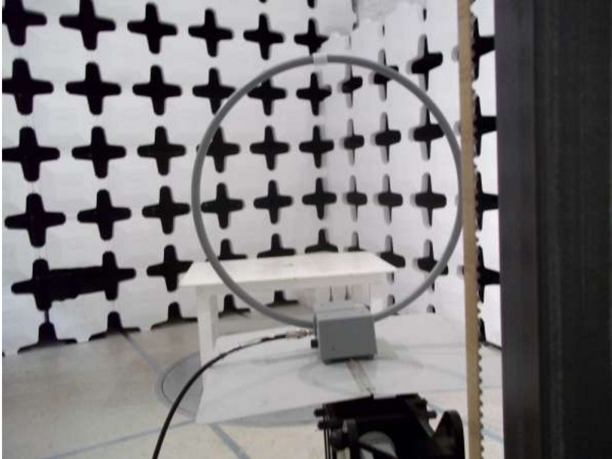
Figure 2. Radiated Emissions Test Configuration (Below 30 MHz)
