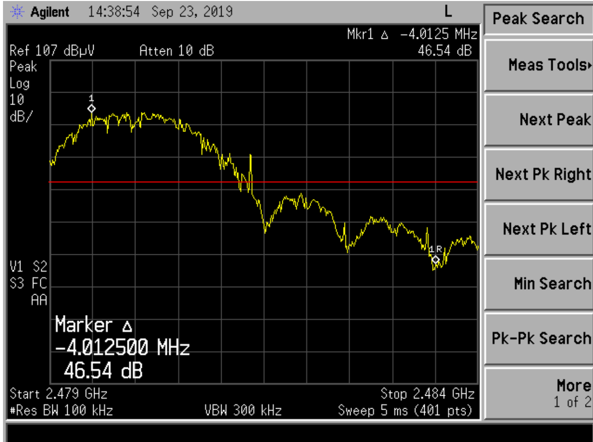
Figure 4. Band Edge Compliance – High Channel Delta
