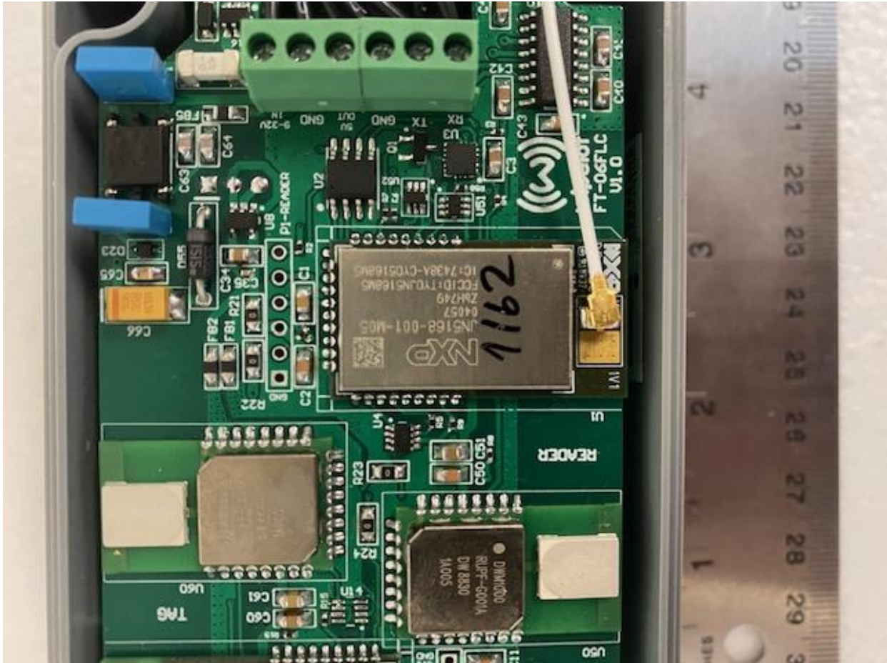
Figure 3. RF Module with Shield
