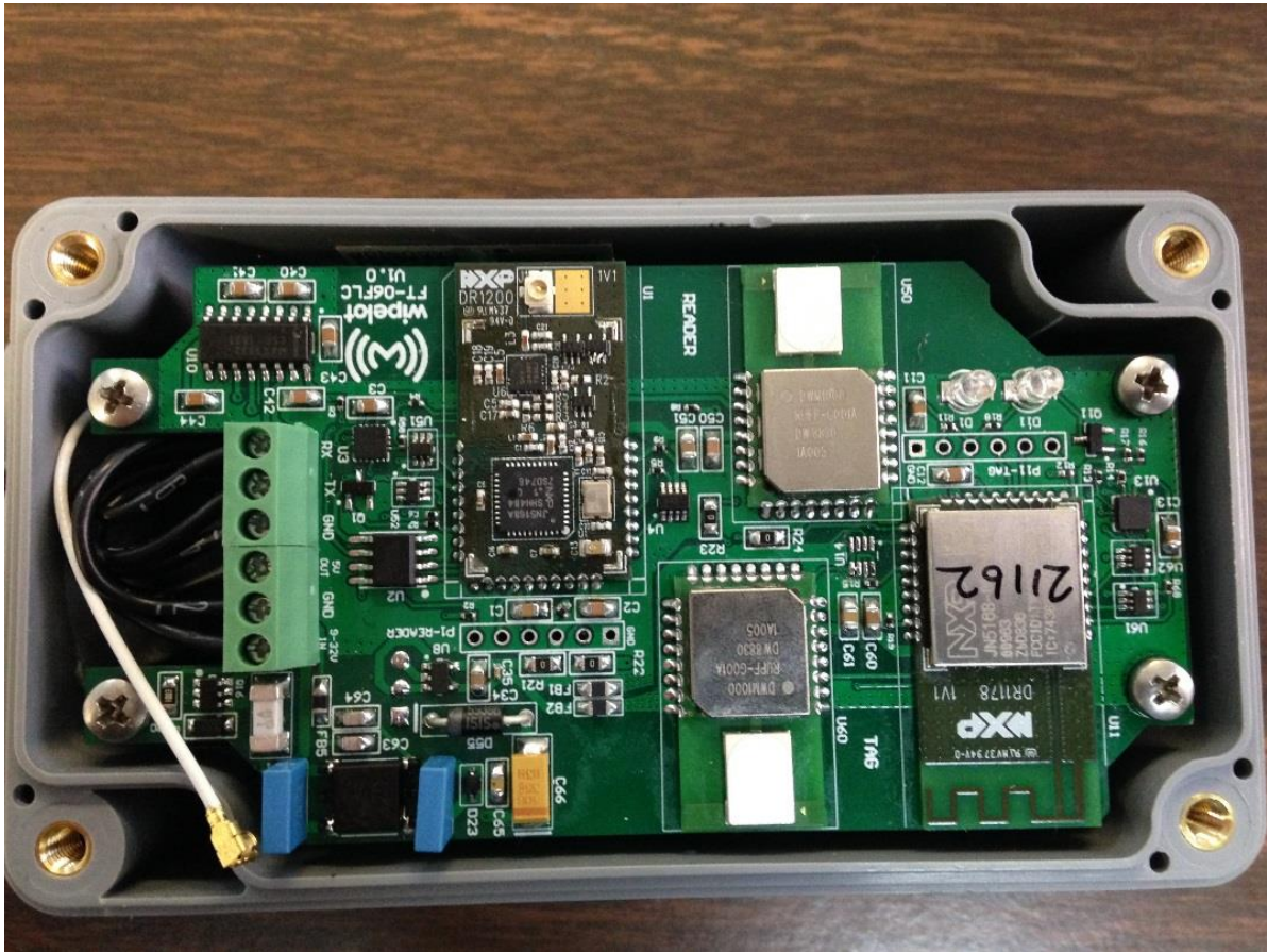
Figure 4. Shield Removed from RF Module
