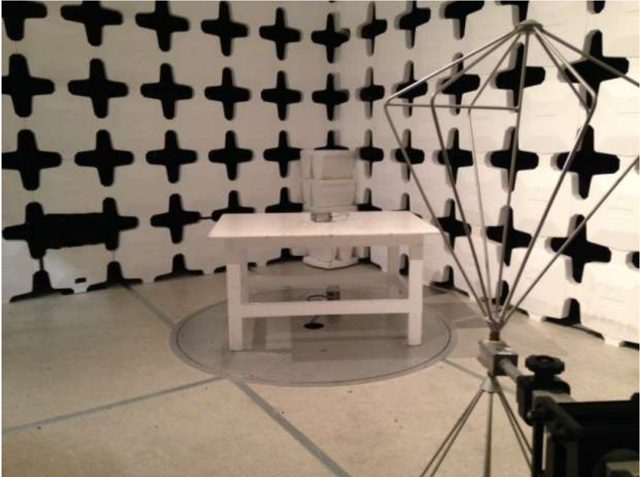
Figure 3. Radiated Emissions Test Configuration (30-200 MHz)
