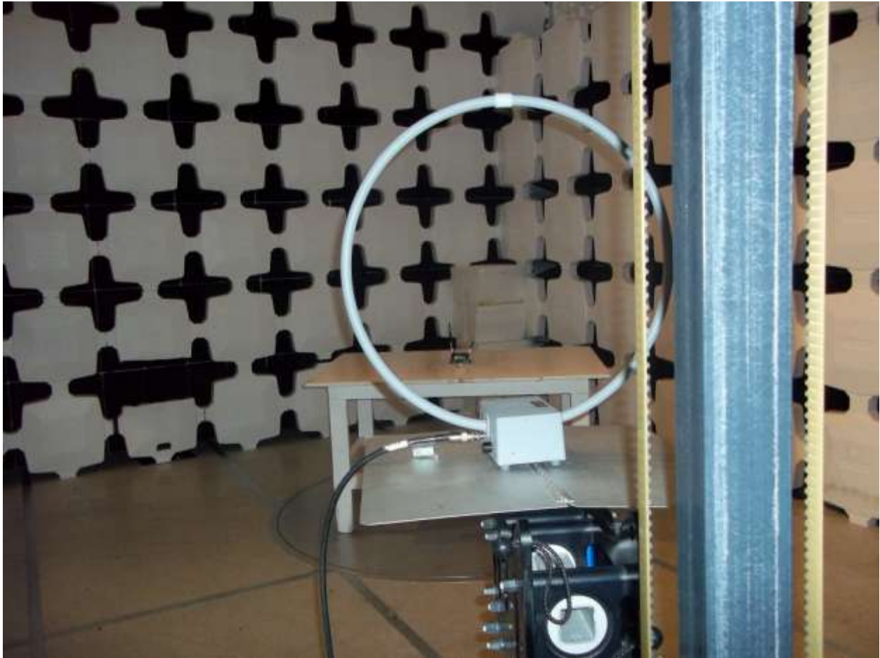
Figure 2. Radiated Emissions Test Configuration (Below 30 MHz)
