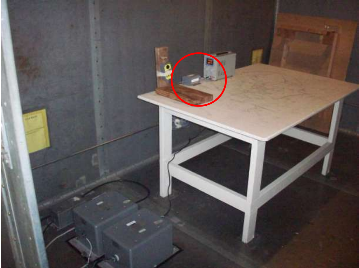
Figure 7. Power Line Conducted Emissions Test Configuration
