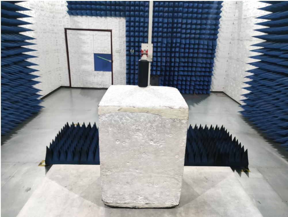
RADIATED EMISSION TEST SETUP ABOVE 1GHz
