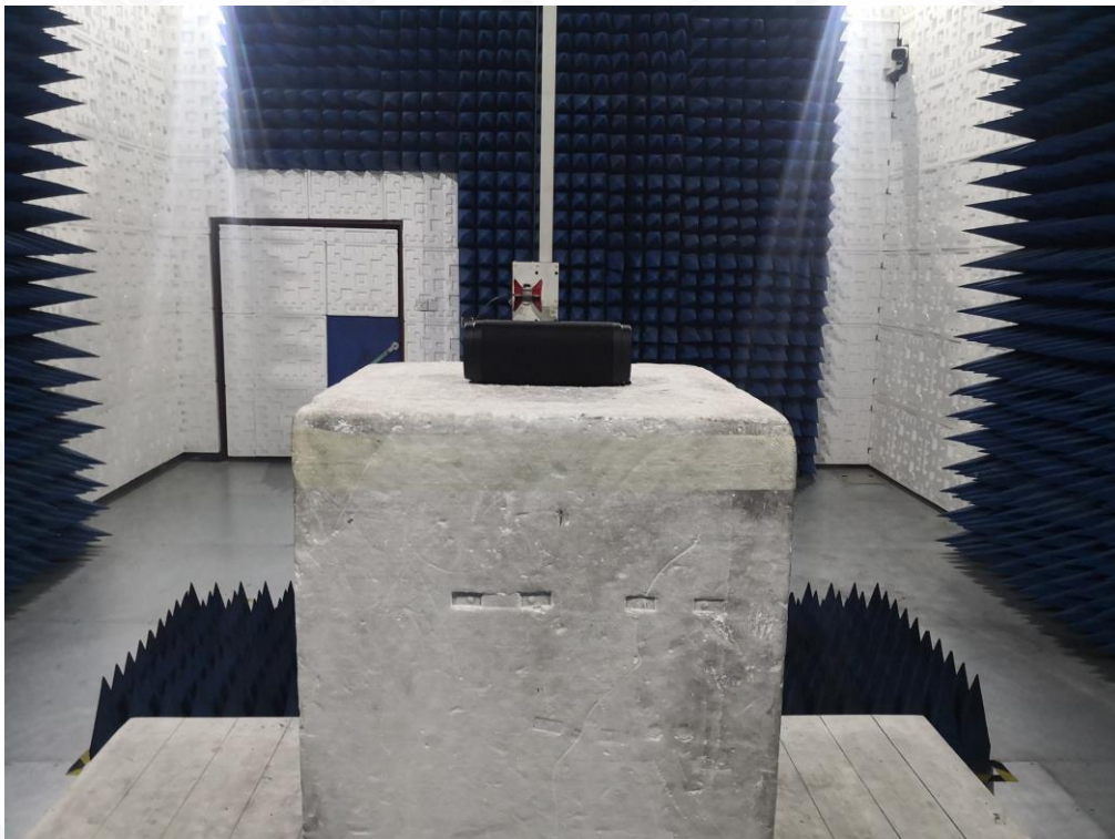
RADIATED EMISSION TEST SETUP ABOVE 1GHZ
