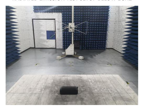
RADIATED EMISSION TEST SETUP ABOVE 1GHZ
