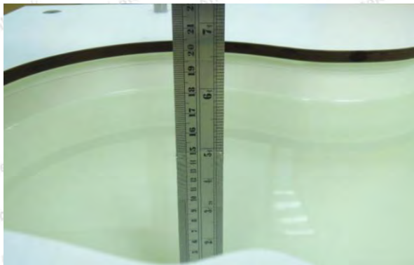
Photo of 1900HSL Liquid Height for Head SAR
