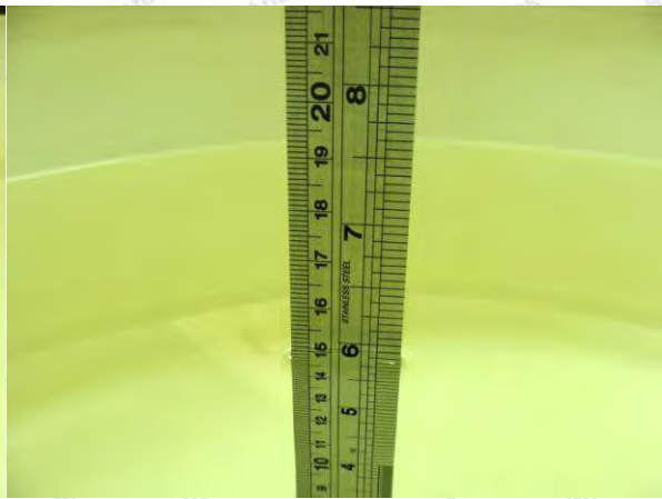
Photo of 900MSL Liquid Height for Body SAR
