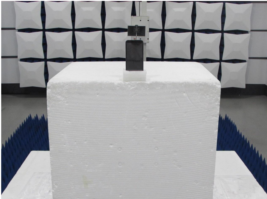
Radiated Emission Above 1GHz
