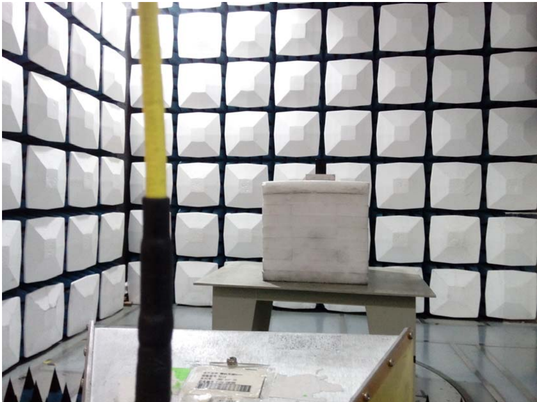
Radiated Emission Above 1GHz View
