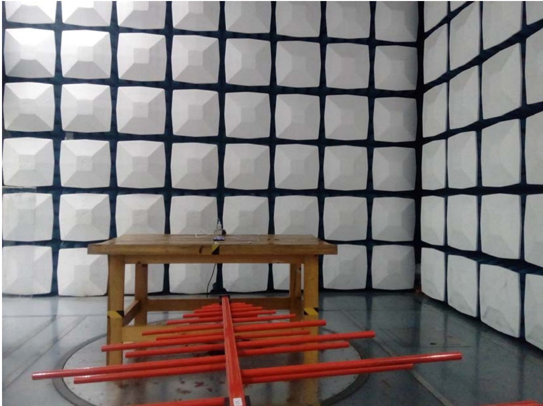
Radiated Emission Above 1GHz View
