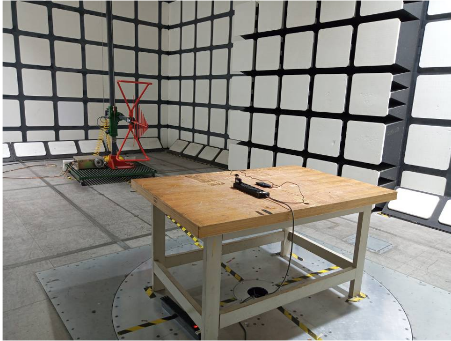
Radiated Emissions View (Below 1 GHz)
