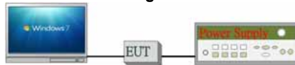
Fig. 2-2 Conducted (Antenna Port) Emission Configuration
