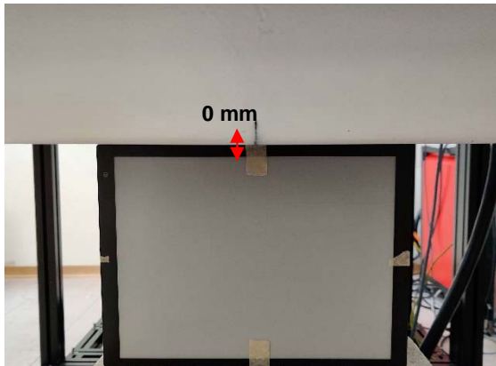
Fig.6 EUT Right side to flat phantom
