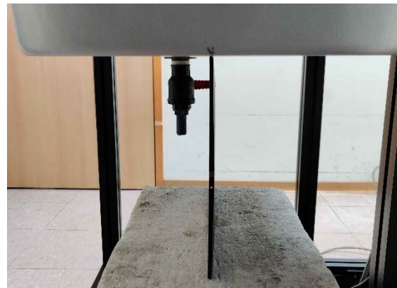
Fig.7 EUT Left side to flat phantom
