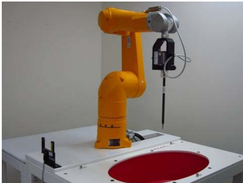
Fig.1 Photograph of the SAR measurement system
