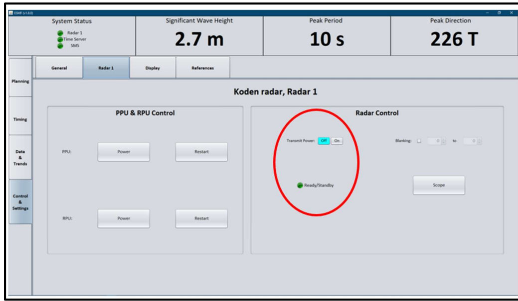
Figure A3: Location of the ‘Transmit Power’ buttons and ‘Ready Status’ indicator in the Radar Control section of the Radar-1 Tab .
