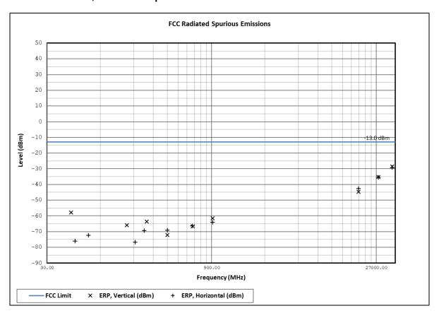
**Note:** All recorded data was plotted. Six (6) or more of the highest emissions of the worst-case operational mode of the EUT are represented below in tabular format. Emissions 20 dB below the limit are not required to be reported.
