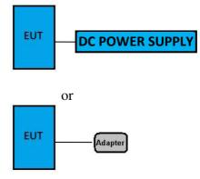
3.9.3. EUT Configuration for RF Conducted Test Items
