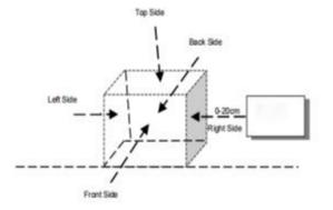
Note: Perform H-field measurements for each edge/top surface of the host/client pair at every 2 cm, starting from as close as possible out to 20 cm
