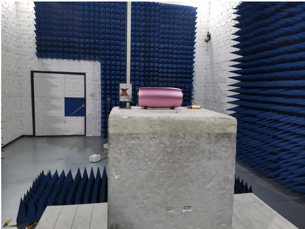
RADIATED EMISSION TEST SETUP ABOVE 1GHZ
