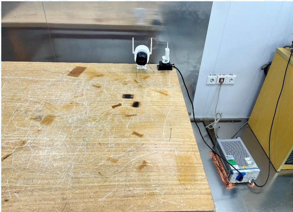
Photo of Setup for Conducted Emission
