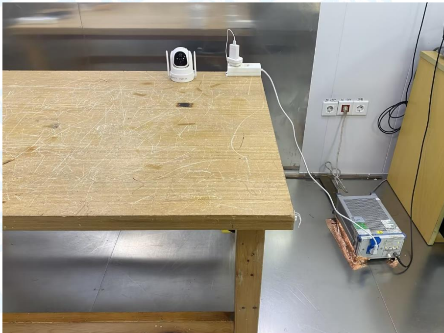
Photo of Setup for Conducted Emission
