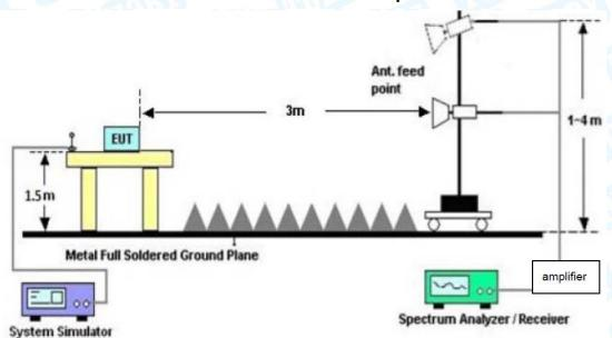
**Above 1GHz Test Setup**
