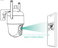
4) After a while, the camera will give out a prompt sound of a successful connection. At this moment, please set the name for the device on the App and select the location you want to place the device. Click "Continue" to complete the pairing.
