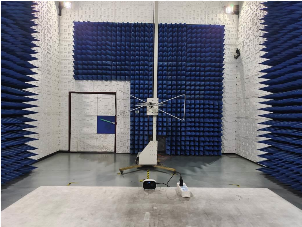
FCC RADIATED EMISSION TEST SETUP ABOVE 1GHZ
