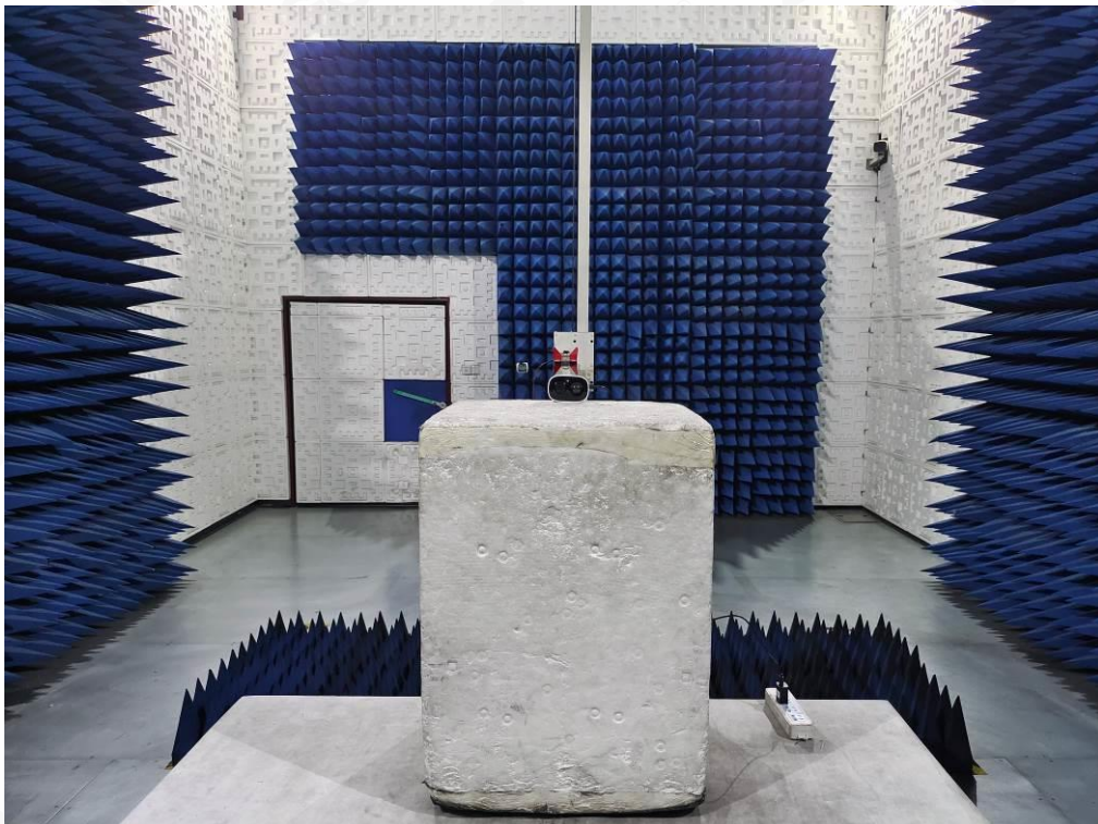
FCC RADIATED EMISSION TEST SETUP ABOVE 1GHZ
