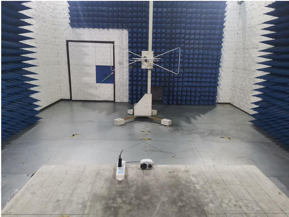
FCC RADIATED EMISSION TEST SETUP ABOVE 1GHZ
