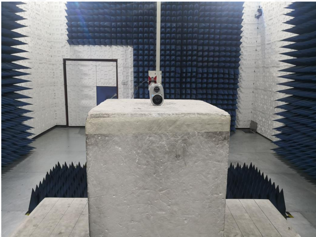
FCC RADIATED EMISSION TEST SETUP ABOVE 1GHZ
