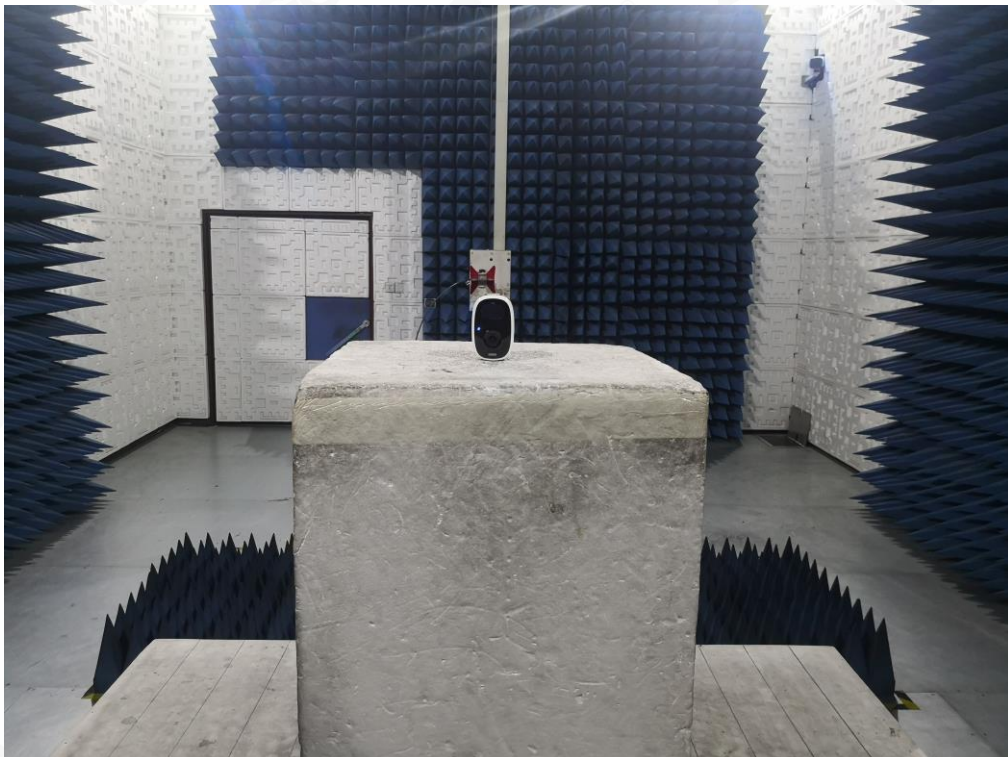
FCC RADIATED EMISSION TEST SETUP ABOVE 1GHZ
