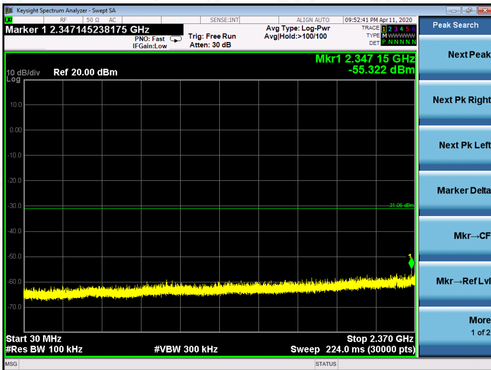
TEST PLOT OF OUT OF BAND EMISSIONS WITH THE WORST CASE OF 802.11g FOR MODULATION IN LOW CHANNEL
