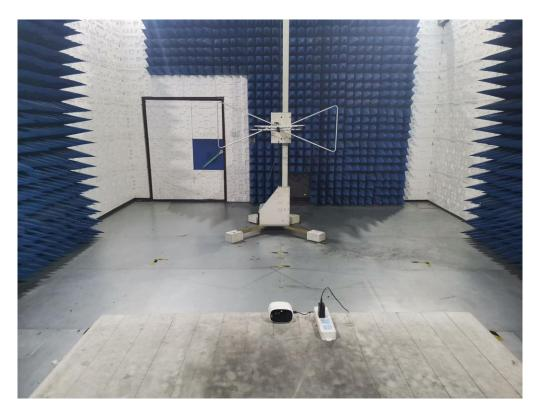
FCC RADIATED EMISSION TEST SETUP ABOVE 1GHZ
