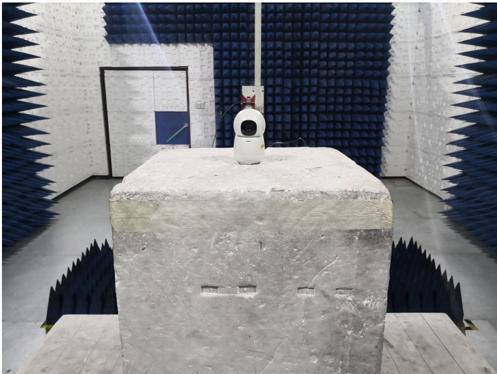
FCC RADIATED EMISSION TEST SETUP ABOVE 1GHZ
