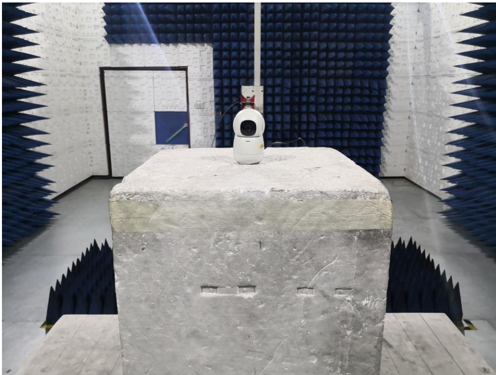
FCC RADIATED EMISSION TEST SETUP ABOVE 1GHZ
