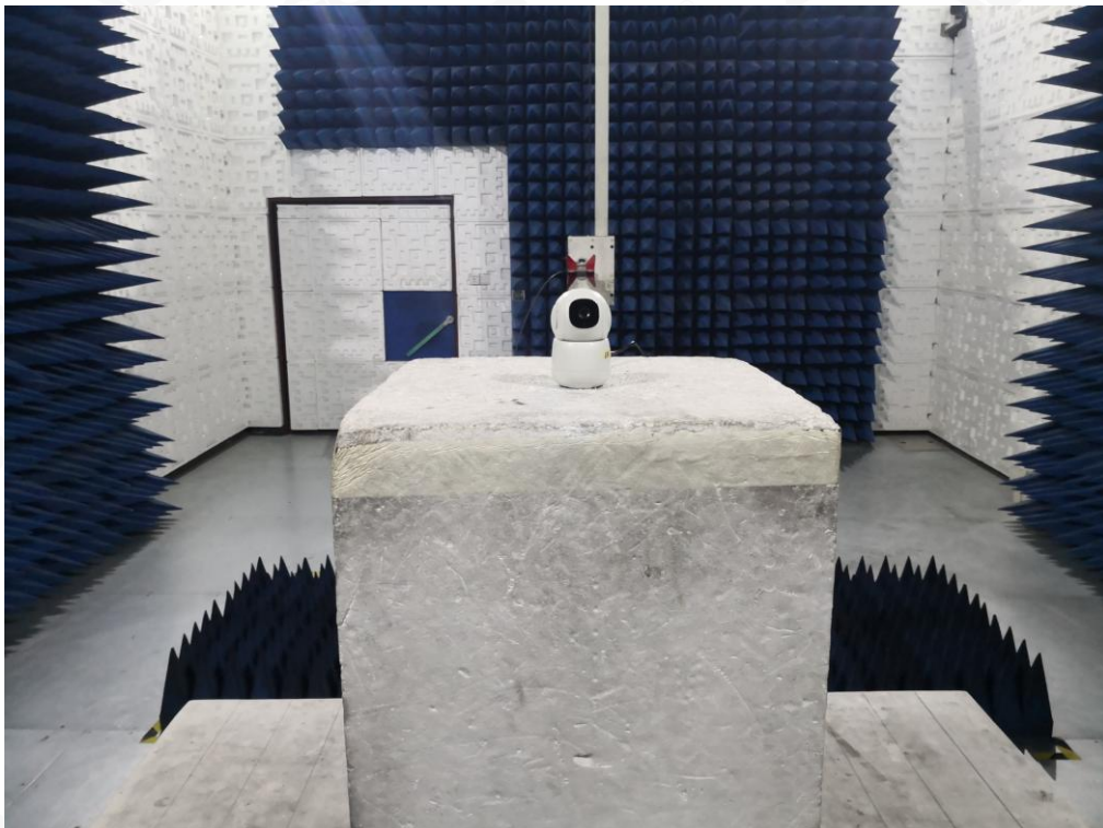
FCC RADIATED EMISSION TEST SETUP ABOVE 1GHZ
