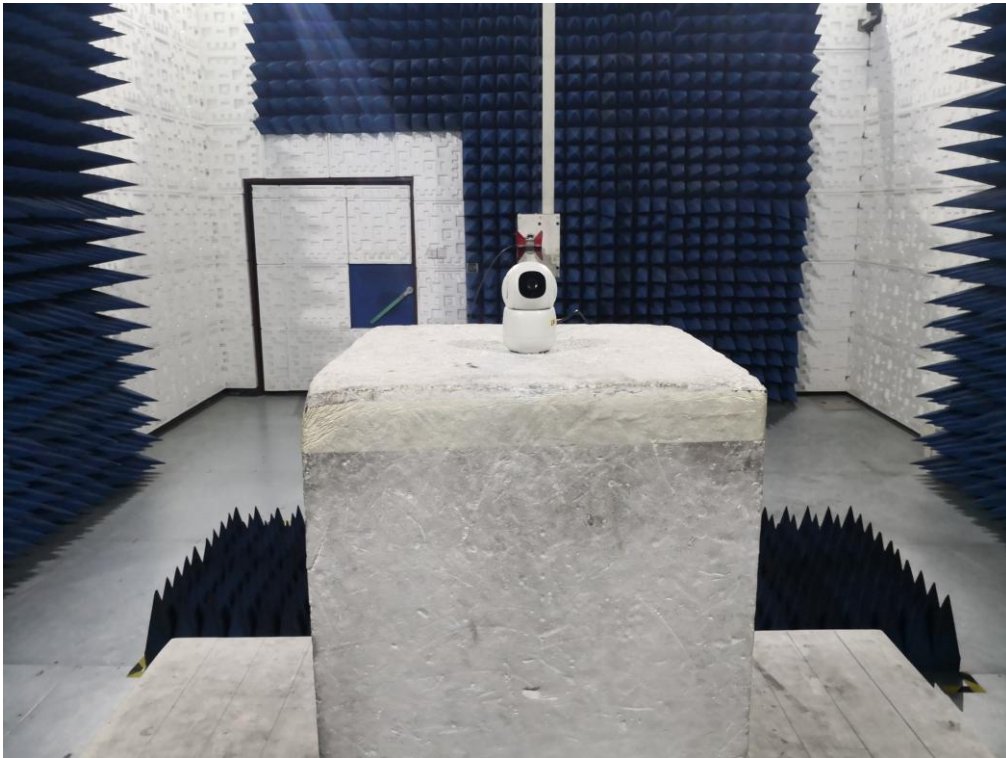
FCC RADIATED EMISSION TEST SETUP ABOVE 1GHZ
