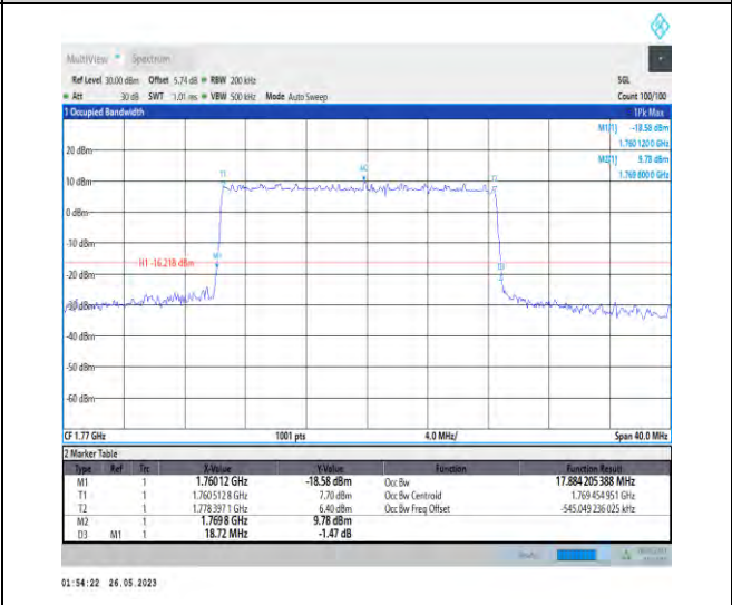
1-N66-PC3-15-20-H-5-DFT-256QAM-Outer_Full-100 @0-17.884-18.720-<=20-PASS
