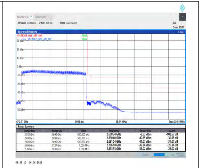
1-N41-PC3-30-100-H-3-DFT-PI2BPSK-Outer_Full- 270@0-Ant1-1--PASS-see graph
