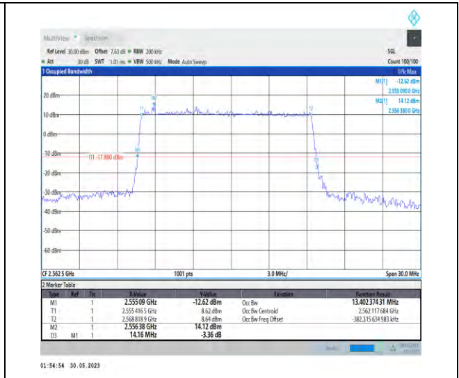
1-N7-PC3-15-15-H-3-DFT-16QAM-Outer_Full-75@0 -Ant1-13.402-14.160-≤15-PASS
