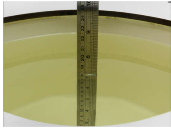
Fig 10.2 Photo of Liquid Height for Body SAR
