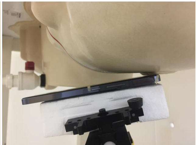
Left Tilted, Test Separation 0 mm
