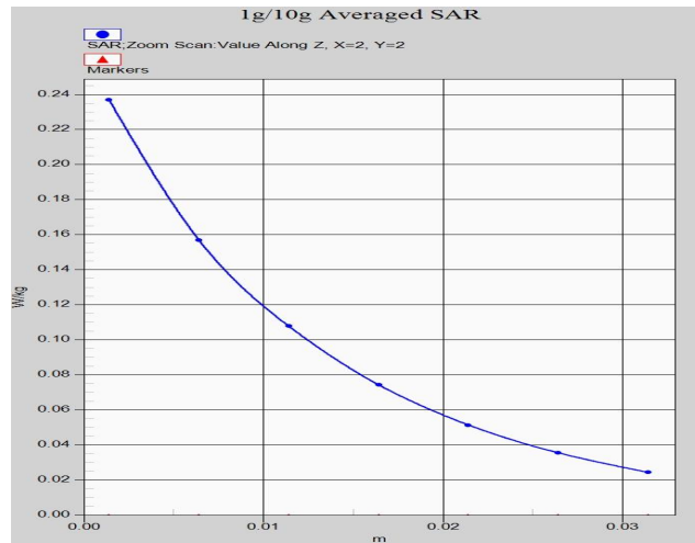
Z-Scan at power reference point (WCDMA1900 ANT31)
