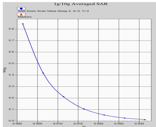
Z-Scan at power reference point (N41 ANT11)
